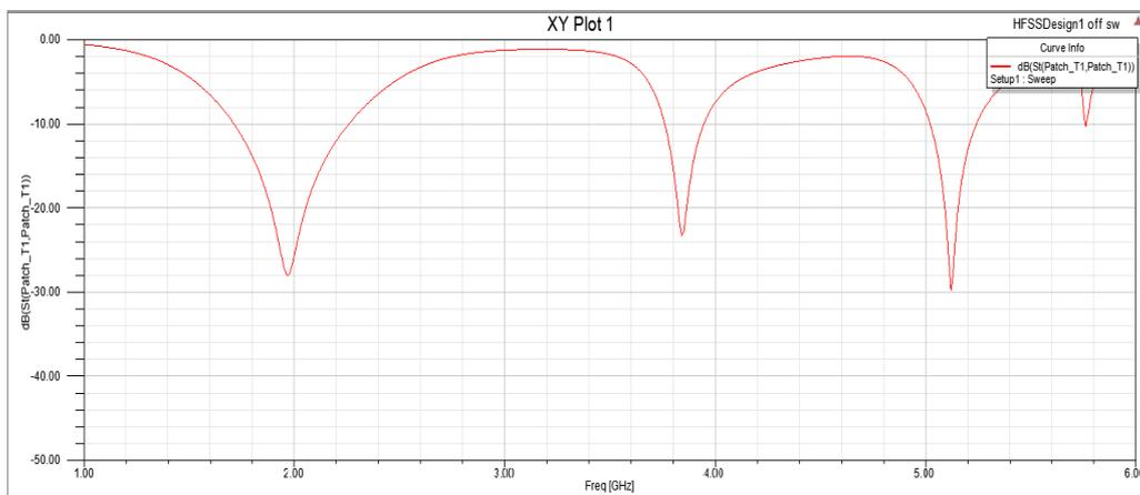
**Figure.2:** Return loss for proposed antenna at switch OFF state
