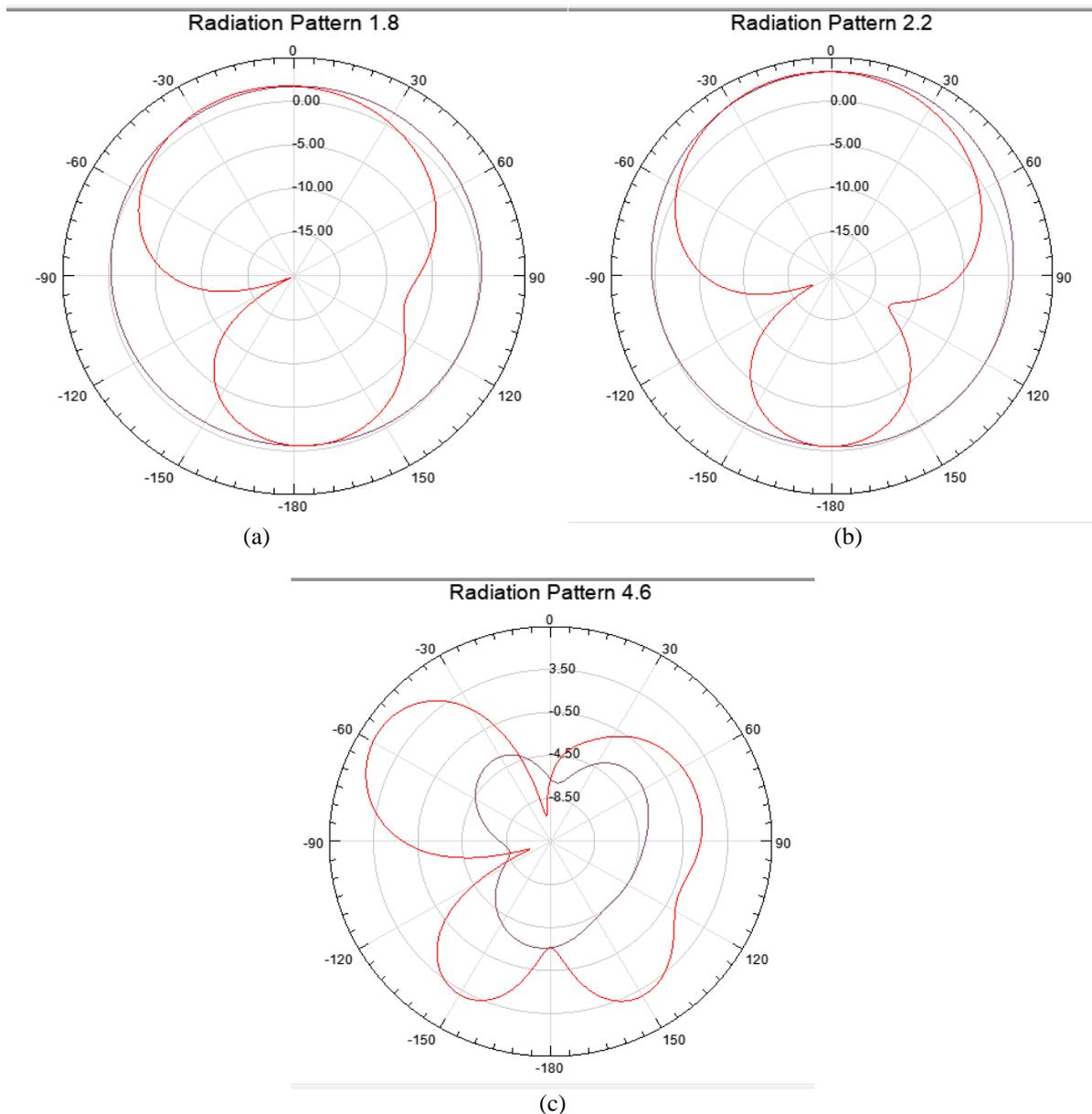
**Figure.5: 2D pattern for the proposed antenna. (a)  $f = 1.8$  GHz, (b)  $f = 2.2$  GHz, (c)  $f = 4.6$  GHz at switch ON condition**
