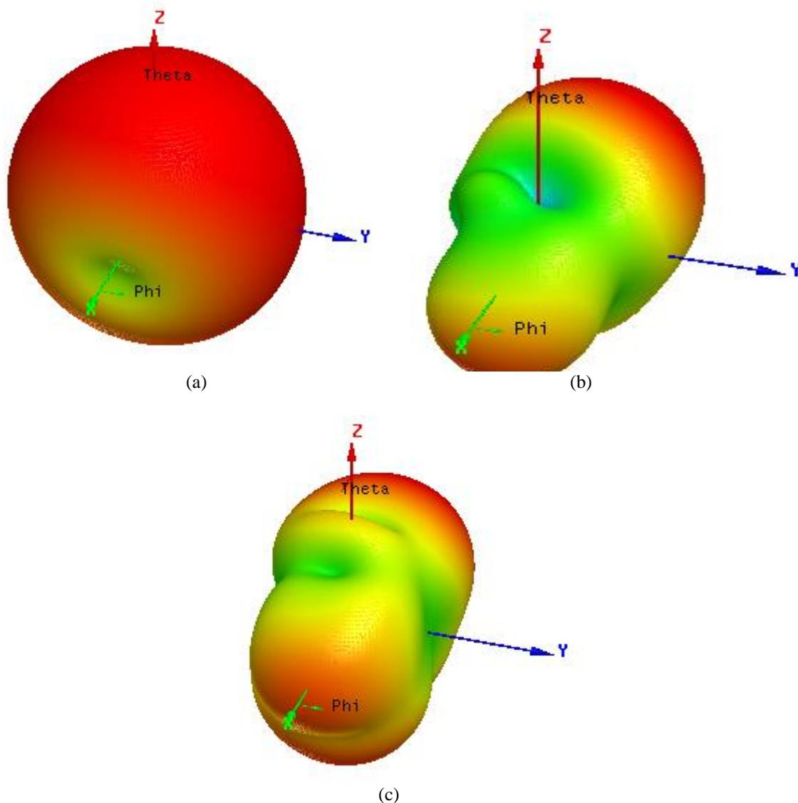
**Figure.6: 3D polar plots for the proposed antenna. (a)  $f = 1.9$  GHz, (b)  $f = 3.8$  GHz, (c)  $f = 5.2$ GHz at switch OFF condition**
