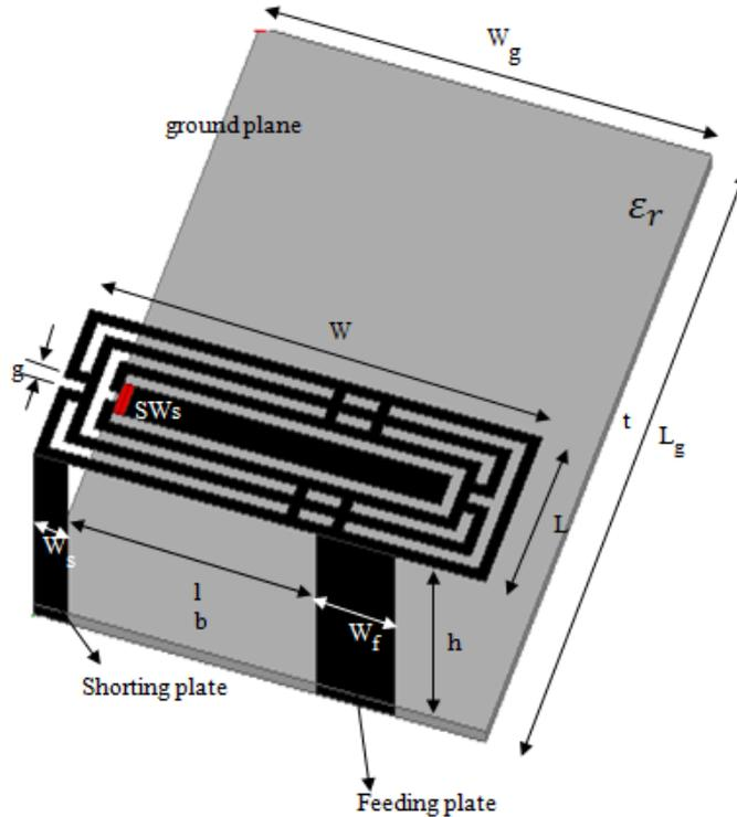
**Figure.1:** Design parameters of proposed antenna:  $W_g = 40$ ,  $L_g = 60$ ,  $W = 40$ ,  $L = 20$ ,  $w_s = 3$ ,  $w_f = 7$ ,  $l_b = 22$ ,  $g = 1$ ,  $h = 10$ ,  $t = 0.64$ ,  $s_1 - s_{12} = 1 \times 1$  (all are in mm),  $\epsilon_r = 6.15$
