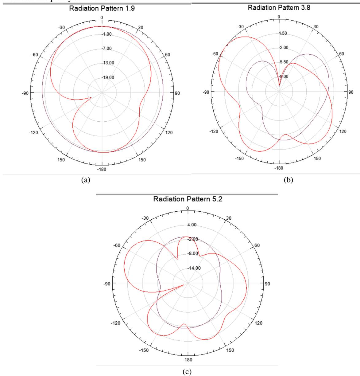
Figure.4: 2D pattern for the proposed antenna. (a)  $f = 1.9$  GHz, (b)  $f = 3.8$  GHz, (c)  $f = 5.2$  GHz at switch OFF condition
