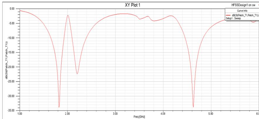
Figure.3: Return loss for proposed antenna at switch ON state
